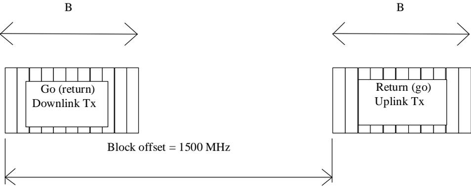
**Figure 3: Application with FDD P-P and P-MP symmetric systems (for one operator)**
