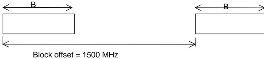
**Figure 1: General concept of paired equal blocks**
