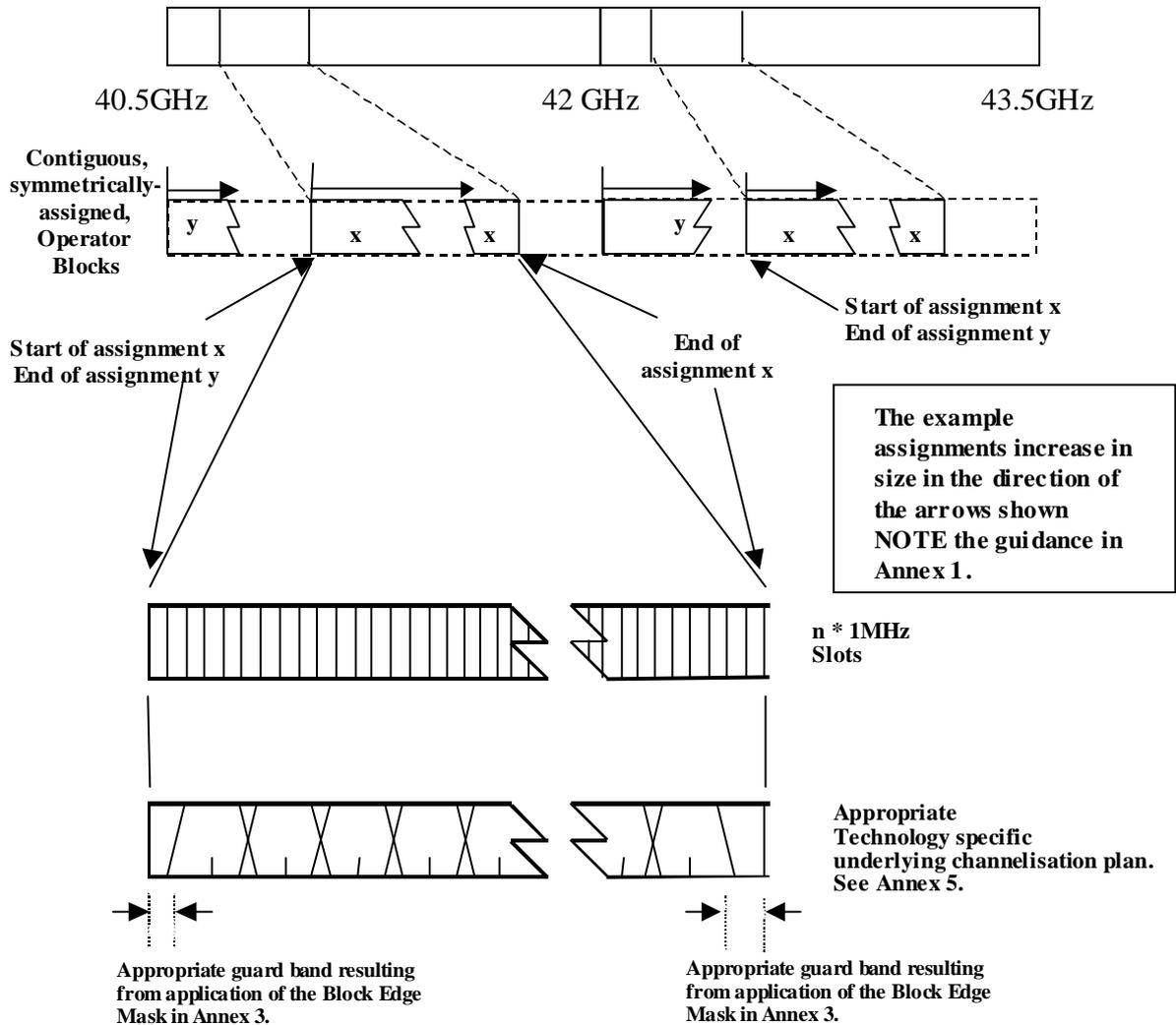
**Figure 8: Frequency plan elements**
