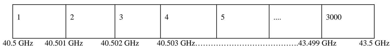
**Figure 7: Basic frequency allocation plan granularity based on 1 MHz slots**
