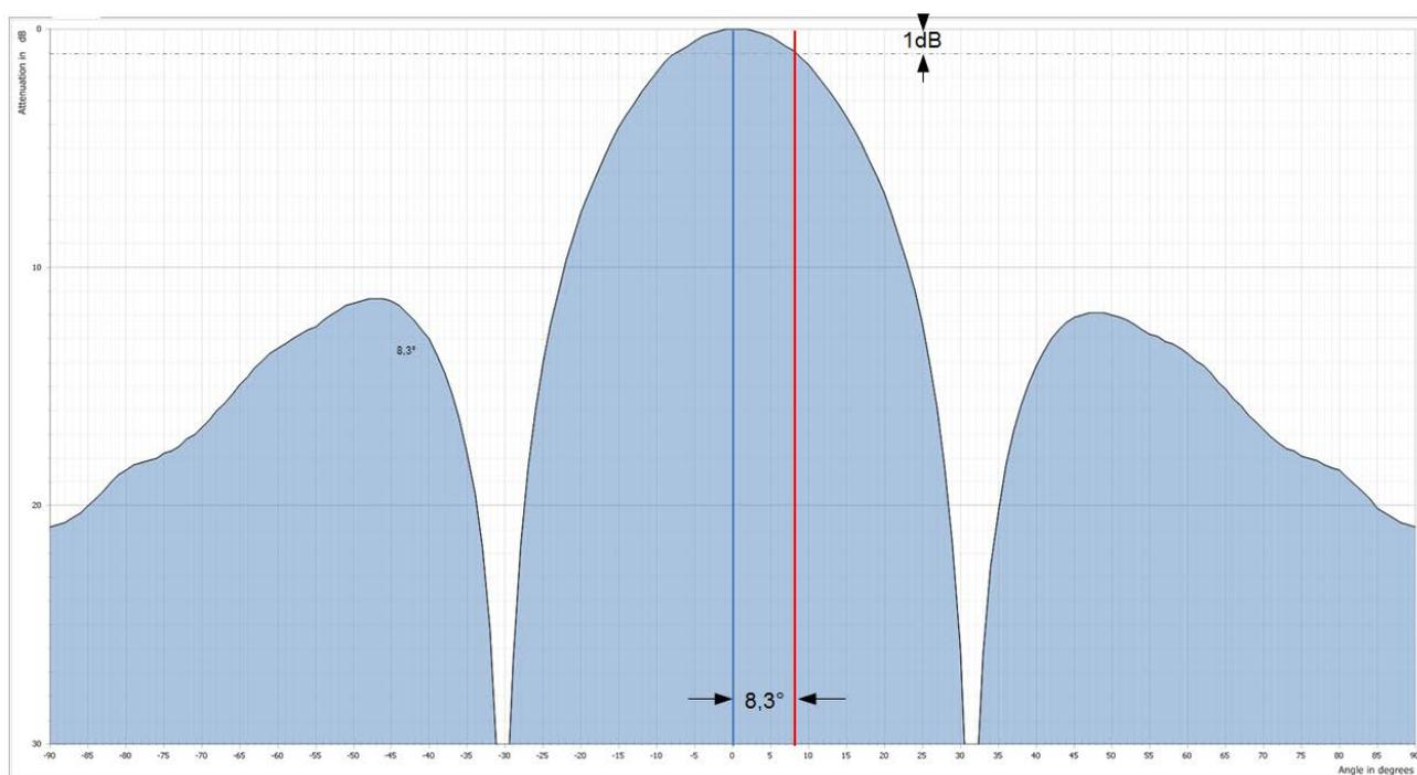
**Figure 5: Determination of the 1 dB angle on a 2-bay antenna**
