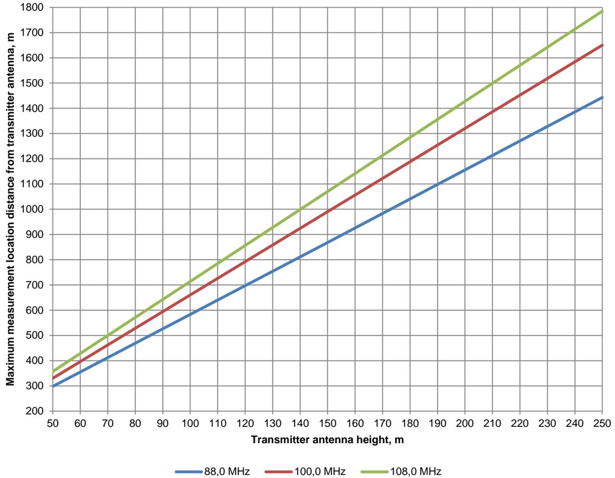
**Figure 4: Determination of the maximum measurement location distance**
