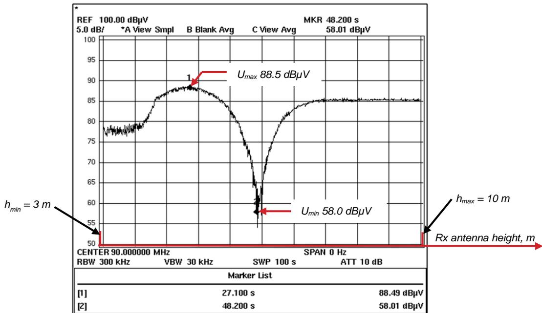
**Figure 2: Example of the dependency of measured signal voltage on measurement antenna height**
