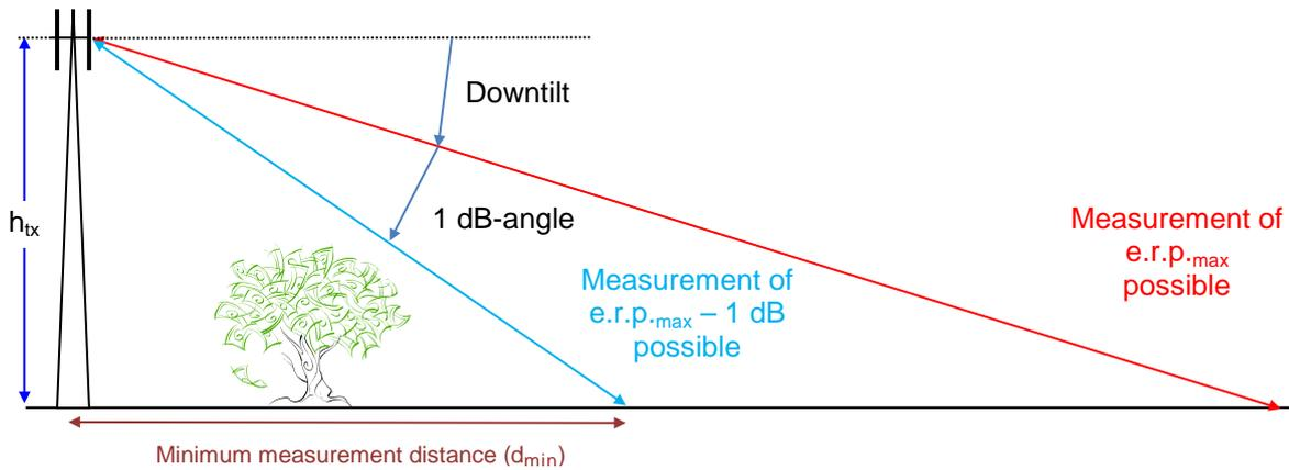
**Figure 6: Determination of the minimum measurement location distance**
